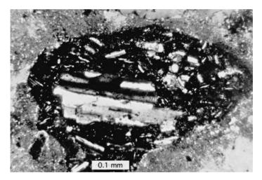
Figure 4.18 Large volcanic clast showing plagioclase laths in a glassy groundmass. Miocene volcaniclastic sandstones, ODP Leg 127, Site 796, Japan Sea (depth 283 m below seafloor). Crossed nicols.
