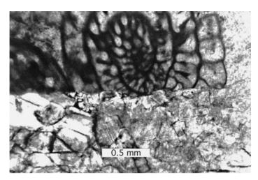
Figure 11.17 Photomicrograph of Fusilinid foraminifer (top) cut in half owing to recrystallization to neomorphic spar (bottom half of photograph). Pennsylvanian limestone, Paradox Basin, Utah. Crossed nicols.
