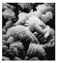
Figure 6.2 Electron micrograph of kaolinite clay minerals magnified 4700 ×. Note the platy or flaky appearance of the pseudohexagonal kaolinite crystals, which are arranged in this specimen in distinct "books."
