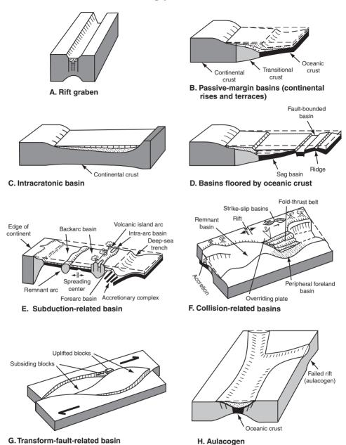
Figure 1.5 Schematic representation of selected kinds of tectonically formed basins. (After Boggs, S., 2006, *Principles of Sedimentology and Stratigraphy*, 4th edn.: Prentice Hall, Upper Saddle River, NJ., Fig. 16.3, p. 556. Reproduced by permission.)
