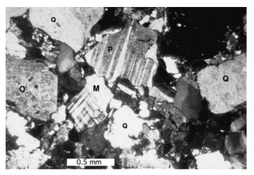
Figure 4.16 Poorly rounded feldspars (M = microcline, O = orthoclase, P = plagioclase) and quartz (Q) in a feldspathic arenite. Belt (Precambrian) facies, Montana. Crossed nicols.
