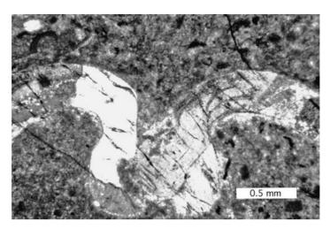
Figure 11.20 Section of a brachiopod shell almost completely replaced by coarse anhydrite. An example of illogical mineral composition as a clue to recognition of replacement fabrics. Pennsylvanian limestone, Paradox Basin, Utah. Crossed nicols.
