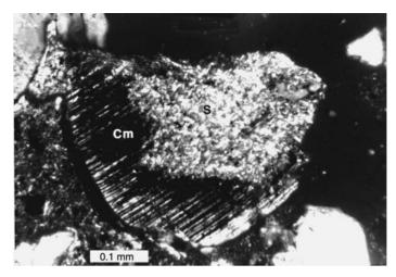
Figure 8.17 Broken, twinned plagioclase grain partially replaced by sericite (S) and dark-colored clay minerals (Cm), Miocene sandstone, Japan Sea. [From Boggs, S., Jr. and A. Seyedolali, 1992, Diagenetic albitization, zeolitization, and replacement in Miocene sandstones, Sites 796, 797, and 799, Japan Sea, in Pisciotto, K. A., J. C. Ingle, Jr., M. T. von Breymann, *et al.* (eds.), *Proceedings of the Ocean Drilling Program, Scientific Results*, vol. 127/128, part 1, Fig. 24, p. 145.]
