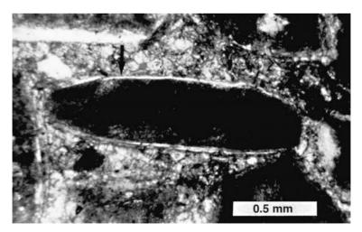
Figure 9.8 Superficial ooid (arrow) that displays a single thin layer or coat around a large micritic nucleus. Tertiary limestone, Spain. Crossed nicols. (Specimen courtesy of P. D. Snavely.)
