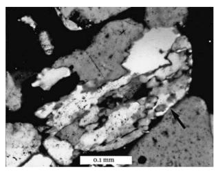
Figure 4.2 Large, well-rounded polycrystalline quartz grain (arrow) that displays sutured internal boundaries between composite crystals, indicating a probable early stage in development of metamorophic polycrystalline quartz. Unknown formation. Crossed nicols.
