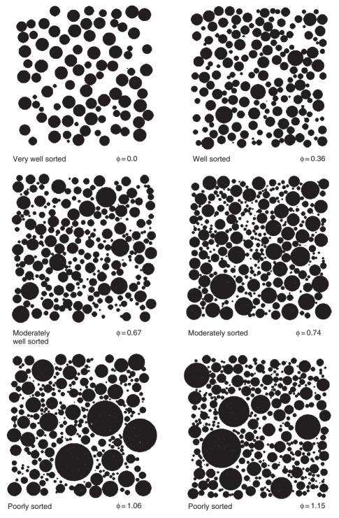
Figure 2.3 Textural comparison chart showing degree of sorting. Each section is labeled with its verbal sorting description according to Folk (1968). (After Jerram (2001), Visual comparators for degree of grain-size sorting in two and three-dimensions: *Comput. Geosci.*, **27**, Fig. 5, p. 490. Reproduced by permission of Pergamon Press, Elsevier Science Ltd.)
