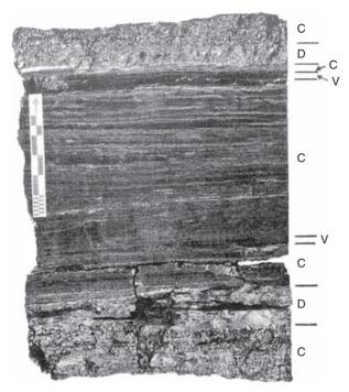
Figure 13.5 Bituminous coal showing examples of three lithotypes: V, vitrain; C, clarain; and D, durain. The small subdivision of the scale = 1 cm. (From Bustin, R. M. *et al.*, 1985, *Coal Petrology, Its Principles, Methods, and Applications*: Geological Association of Canada Short Course Notes 3, Pl. 6A, p. 51, reprinted by permission.)
