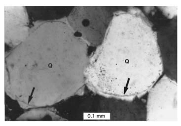
Figure 4.14 Photograph of two quartz grains (Q) with overgrowths. Note that original grain outlines are clearly marked by a line of impurities (arrows) and that the grain on the right is almost completely surrounded by the overgrowth. Quartz arenites of the Deadwood Formation (Cambrian–Ordovician), South Dakota. Crossed nicols.
