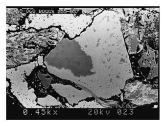
Figure 8.18 Partially albitized plagioclase grain (center of photograph), as revealed by backscattered electron microscopy (BSE). The dark patches are albitized areas. Miocene deep-sea sandstone, Japan Sea. Ocean Drilling Program Leg 127, Site 797. (Photograph courtesy of David Krinsley.)
