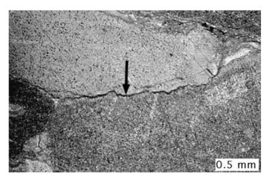
Figure 11.10 Sutured contact or microstylolite (arrow) between two crinoid fragments, formed as a result of pressure solution (chemical compaction), Middle Mississippian limestone, Oklahoma.
