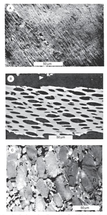
Figure 13.6 Examples of coal macerals, as illustrated in reflected-light photographs: A – telinite, a vitrinite maceral; B – fusunite, an inertinite maceral; and C – resinite (R), a liptinite maceral. (After Bustin, R. M. *et al.*, 1985, *Coal Petrology, Its Principles, Methods, and Applications*: Geological Association of Canada Short Course Notes 3., Pl . 3, Fig. 5, p. 41; Pl. 4, Fig. 2a, p. 45; Pl. 5, Fig. 1, p. 47, reprinted by permission.)
