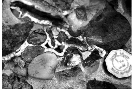
Fig. 18.18 An isopachous, sparry calcite cement formed in the pore spaces between pebbles lines the surfaces of the pebbles.
