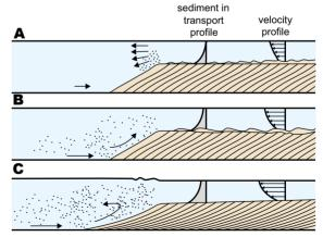
**Figure 6.48** The changes in shape of the slip face of a small laboratory delta due to progressive increase in the velocity of flow over it from A to C. After Jopling (1965).
