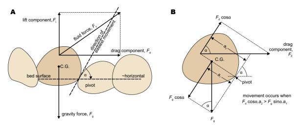
Figure 3.17 A) The forces acting on a particle in a bed of similar particles when subjected to the shear of an over-riding current. B) The movement forces which must be balanced for incipient motion; movement begins when  $F_{\rm d}$   $a_{\rm g}$  cos  $\alpha > F_{\rm g}$   $a_{\rm q}$  sin  $\alpha$ . C.G. is centre of gravity. After Middleton and Southard (1977, 1984).
