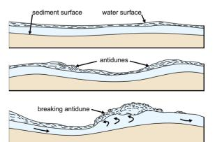
**Figure 6.67** Development of standing waves and antidunes as observed in a laboratory flume experiment. Note how the water and sediment waves are in phase with one another and how the antidunes break in an upstream direction. Each section is 1m long. Modified after Kennedy (1961).
