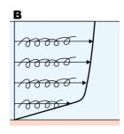
Figure 3.3 Vertical velocity profiles for A) laminar and B) turbulent flows in an open channel of great width. In the profile for turbulent flow, the velocities are time-averaged values and only close to the bed does a near-laminar pattern of movement occur.
