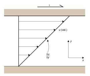
**Figure 3.1** Definition diagram for viscosity. Two rigid parallel plates enclose the fluid. A shear stress  $(\tau)$ , acting parallel to 'sheets' within the flow sets up the steady-state velocity profile shown by the inclined line. The length of the arrows is proportional to velocity (u) relative to the lower plate.
