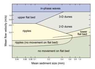
**Figure 6.22** The stability fields of different bedforms in relation to flow velocity and grain size for water depth of 0.2m. Note that the plot is on a log-log scale. For other depths, the position of the lines are shifted and a three-dimensional plot is needed to illustrate fully the bedform distribution. After Harms et al. (1975).
