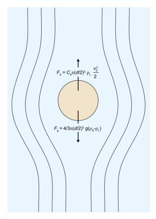
**Figure 3.14** The forces acting on a spherical particle falling through a fluid. The streamlines indicate that flow around the particle is laminar and therefore either the viscosity of the fluid is high or the particle is small.
