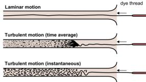
**Figure 3.2** The Reynolds experiment to illustrate the difference between laminar and turbulent flow. Dye injected into the flow from a point source behaves in different ways depending on the velocity and viscosity of the flowing fluid. After Allen (1968).
