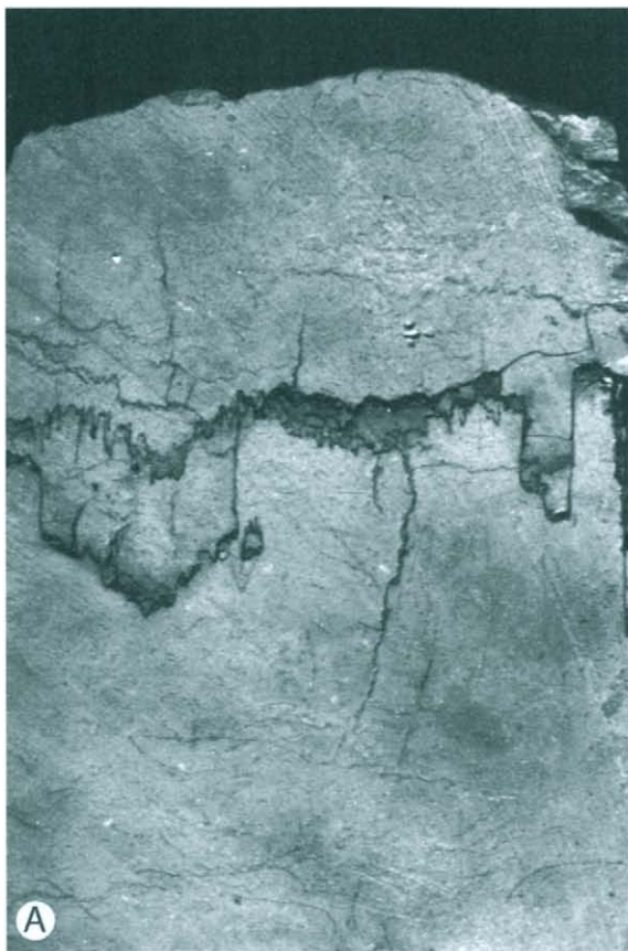
Fig. 9.9. (A) A 6-cm-diameter core of Paleocene limestone with stylolites due to solution. Sirte basin, Libya. (B) Sketches illustrating how to measure the amount of vertical displacement due to stylolitic solution.
