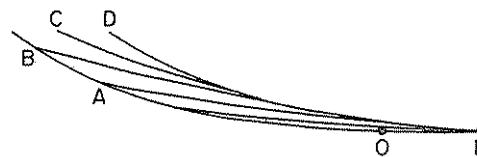
Fig. 11.11. Fluvial aggradation due to shift of stream equilibrium profile from O (original point of grade), with initial profile AO, to F (final point of grade). According to Posamentier et al. (1988) the river aggrades in response to this shift, developing in turn profiles BF, CF, and DF (letters added to original illustration of Posamentier et al. 1988, Fig. 15). (Diagram from Miall 1991c)
