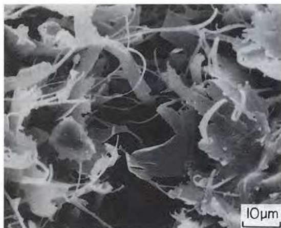
Fig. 2.54 Scanning electron micrograph of authigenic illite in the form of radially arranged flakes and whiskers growing into pore space between two sand grains (left and right of picture). Rotliegend desert sandstone, Lower Permian. Northern Germany.
