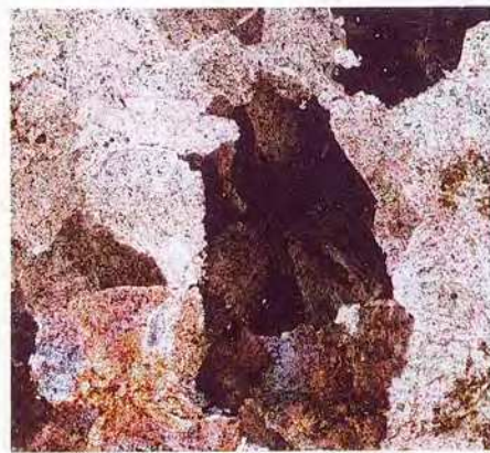
(e) Dolomite moulds: grainstone with scattered dolomite rhombs that have been dissolved out to give a good porosity, as shown by blue resin. Stylolitic contacts between grains. Jurassic. Burgundy, France. Field of view 0.8 \times 0.8 mm.
