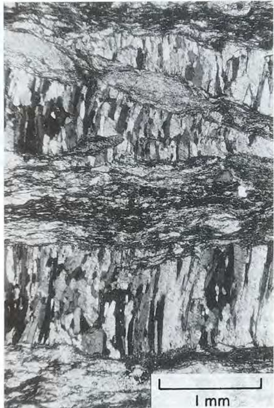
Fig. 5.9 Veins of fibrous gypsum ( satin spar ) in gypsiferous mudrock. Crossed polars. Permian. Cumbria, England.
