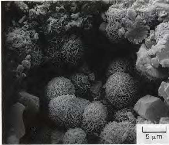
Fig. 9.7 Lepispheres of opal-CT growing in voids in silicified Eocene chalk from the Arabian Sea. Sample from 630 m below sea floor. Prismatic crystals are clinoptilolite (a zeolite). Scanning electron micrograph.
