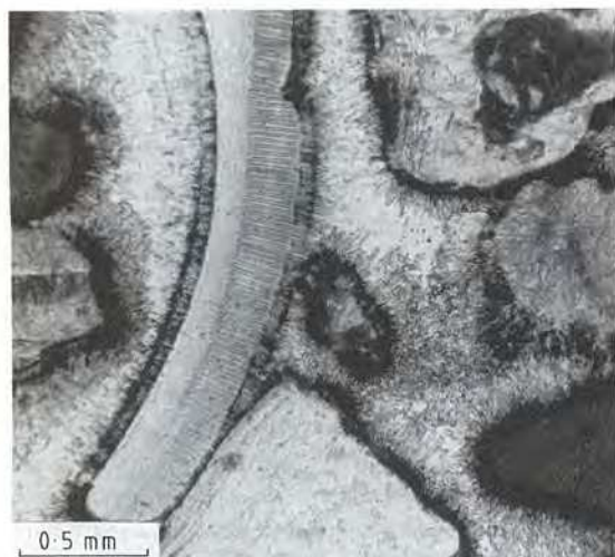
Fig. 4.28 Beachrock with cements of acicular aragonite and micritic high-Mg calcite: the latter is the dark coating around grains. The aragonite cement has grown syntaxially on the bivalve grain, which shows a two-layer shell structure. Plane polarized light. Great Barrier Reef, Australia.
