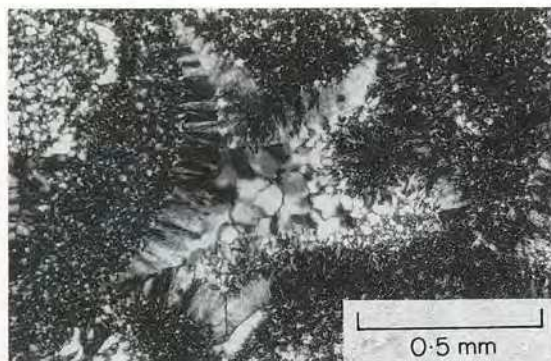
Fig. 9.1 Photomicrograph showing: microquartz—finely crystalline mosaic with pin-point extinction; megaquartz—larger quartz crystals in central part; chalcedonic quartz—in a fibrous fringe. In this case, the microquartz is a replacement of carbonate grains and the megaquartz and chalcedonic quartz are pore filling. Crossed polars. Carboniferous. Glamorgan, Wales.
