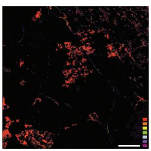
Figure 24.8: A Ca<sup>2+</sup> BSE elemental map from the area in Figure 24.7. Most of the red areas represent calcite cements. Scale bar = 0.3 mm. Highest concentrations are red and lowest are violet.
