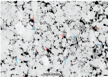
Figure 24.14: A shale sample imaged with an SEM at a resolution of 10 nm/pixel. Porosity (red arrows) is associated with organic matter (blue arrows) in a predominantly quartz matrix. The image aids in understanding the distribution of the porosity and organics in shale, and allows computation of poresize distribution. Scale bar = 1  $\mu$ m.
