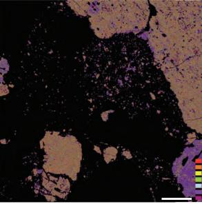
Figure 24.9: A Na<sup>+</sup> BSE elemental map of the area in Figure 24.7. The sodium distribution marks the location of albite replacements (orange color) and an original albite grain (purple color). Scale bar = 0.3 mm. Highest concentrations are red and lowest are violet.
