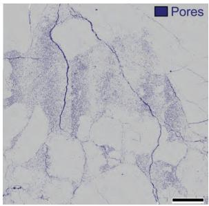
Figure 24.11: A map of pore distribution in the area from Figure 24.7. Scale bar = 0.3 mm.
