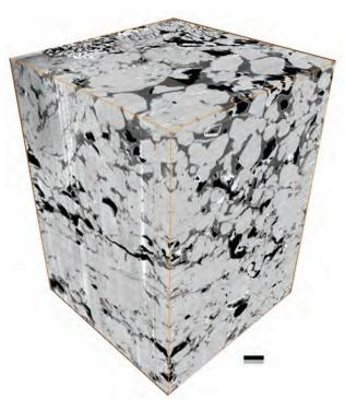
Figure 24.16: A high-resolution 3-D FIB-SEM volume. Pores (black) are associated with organic matter (dark gray) and the mineral matrix (light gray). Absolute permeability is calculated in the x, y, and z directions. Scale bar = 1  $\mu$ m.
