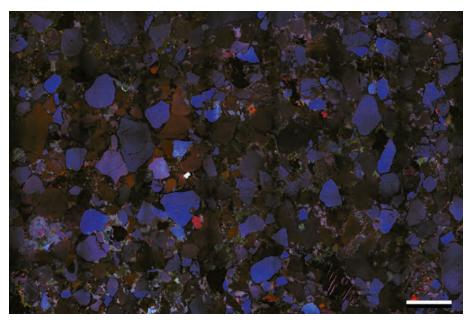
Figure 24.2: Large areas of a sandstone can be viewed with color CL on an SEM and the multiple images can be stitched together with software. Scale bar =  $367 \mu m$
