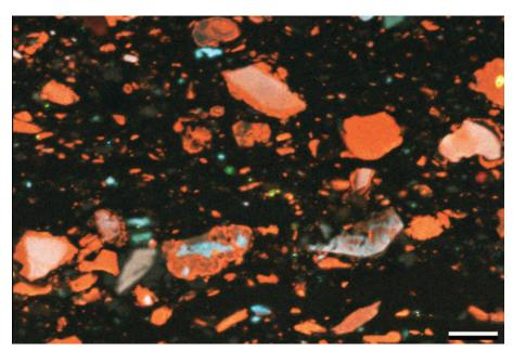
Figure 24.4: Silt-size quartz grains from the Up. Devonian New Albany Shale, Indiana. In scanned color CL a wide range of different types of quartz grains is apparent. Many have interior cores that indicate previous episodes of sediment recycling, from sources that are plutonic as well as metamorphic. Some grains show nonluminescent diagenetic overgrowths, followed by later diagenetic (higher temperature, reddish) overgrowths. Scale bar =  $14 \mu m$
