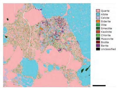
Figure 24.7: A mineral map of the of the area shown in Fig. 24.6. The reddish brown areas in Fig. 24.6 that might easily be mistaken for K-feldspar are actually albite-replaced K-feldspar (blue areas in this figure). Scale bar = 0.3 mm.
