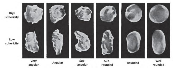
Figure 6.3: A visual comparator showing levels of rounding in high and low sphericity sand grains (from Powers, 1953).
