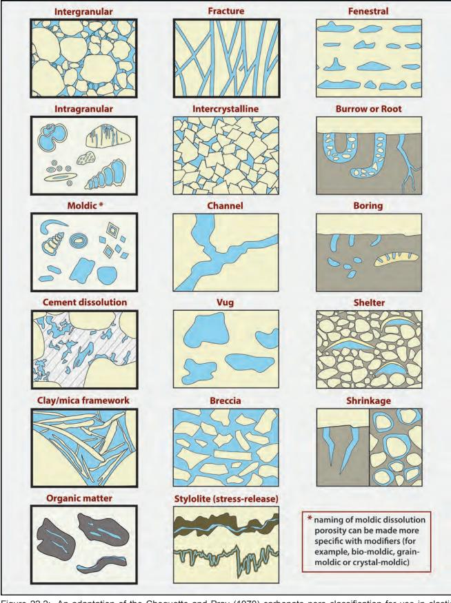
Figure 22.2: An adaptation of the Choquette and Pray (1970) carbonate pore classification for use in clastic terrigenous rocks. A number of categories have been dropped and some new ones added, including clay framework and organic matter pore types that are especially important in mudrocks (Loucks et al., 2012 and Schieber, 2013). Although all these pore types can occur in clastic terrigenous and associated rocks, those outlined with a darker box are most the common ones.
