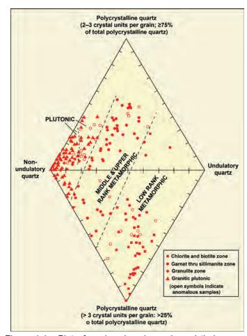
Figure 1.1: Plot of modern beach sands and their source terranes shows how the amount of nonundulatory, undulatory and polycrystalline quartz grains and the number of crystals in polycrystalline grains can help determine quartz provenance (from Basu et al., 1975).
