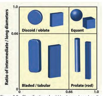
Figure 6.2: Classification of pebble shapes based on the relative lengths of their three mutually perpendicular axes. Adapted from Zingg (1935) and Krumbein (1941).
