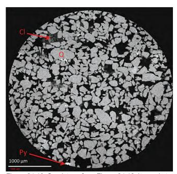
Figure 24.13: Sandstone from Figure 24.12, imaged at a resolution of 4  $\mu$ m/voxel using a MicroCT scanner. Note as resolution increases, field of view decreases. At this resolution, sparse clay (Cl), which appears dark gray but lighter than pores, can be seen between quartz (Q) grains. High-density pyrite (Py) clusters are present.
