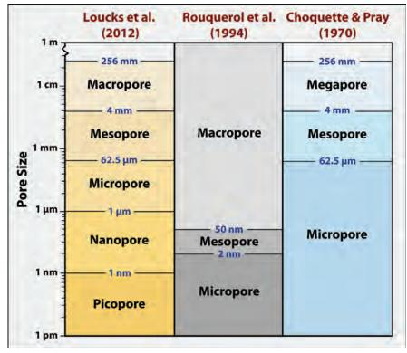
Figure 22.1: A comparison of three terminological schemes for pore sizes in sedimentary rocks and other porous solids. Sizes measurements are typically based on the diameter of circular pores or the width of elongate pores. Adapted from Loucks et al. (2012).
