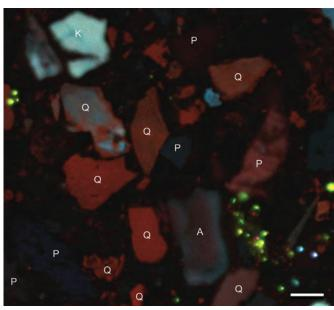
Figure 24.3: Low- and medium-grade metamorphic grains in the Cretaceous Mancos Shale (Utah) that were derived from the Sevier Orogenic belt (Q = quartz, P = plagioclase, K = K-feldspar, A = albite). Scale bar = 10.5  $\mu \rm m$
