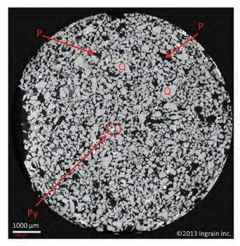
Figure 24.12: A relatively pure quartzarenite sample imaged using the MicroCT scanner. Single axial image above has a resolution of approximately 8  $\mu$ m/voxel. Scan is based on density, therefore pores (P) appear dark (near black) and grains light gray. In this scan almost all grains are quartz (Q). Small, high-density pyrite (Py) clusters are present.
