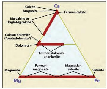
Figure 15.1 A diagram showing the general compositions of carbonate minerals found in modern and ancient rocks.
