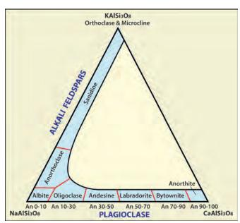
Fig. 2.1: Ternary feldspar compositional diagram.
