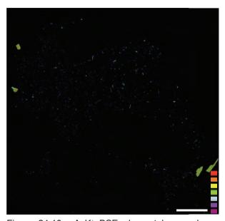
Figure 24.10: A K+ BSE elemental map shows little potassium in the sample area, therefore no orthoclase or K-feldspars. The green areas are muscovite grains. Scale bar = 0.3 mm. Highest concentrations are red and lowest are violet.
