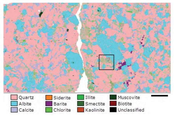
Figure 24.5: A mineral map of the entire Up. Pennsylvanian Bursum Fm. thin section showing the distribution of mineral phases. Based on the outcrop samples, the sample was thought to comprise mostly quartz and potassium feldspars. Based on analysis, however, it was shown that quartz (pink) and albite (pale blue) dominate. Scale bar = 4.8 mm.
