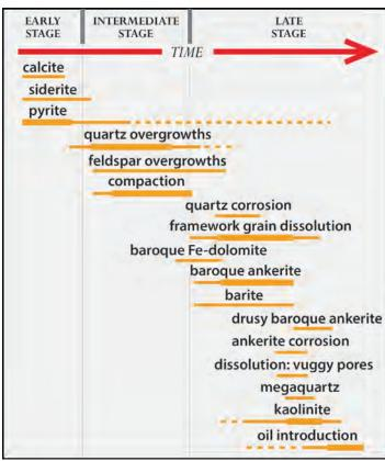
Figure 23.1 A summary paragenetic sequence for Pennsylvanian sandstones of the Cherokee Basin in Kansas showing diagenetic events and their relative (and extensively overlapping) timing. The thicknesses of the lines reflect the relative intensity of processes through time and dashed lines indicate the possible range over which a given alteration may have occurred. The data are based on petrographic, geochemical and fluid-inclusion studies. Adapted from Wojcik et al. (1997, p. 237).
