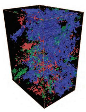
Figure 24.17: A high-resolution, segmented 3-D FIB-SEM cube where green represents organic matter, blue is connected porosity, and red is isolated porosity.
