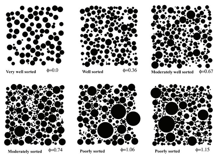
Figure 6.1: Six textural comparators for degree of sorting in 2-D. Each comparator is labeled with its sorting description (Folk, 1968) based on the true 3-D sorting value. Adapted from Jerram (2001).
