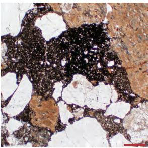
Figure 24.6: A plane-polarized light view of the thin section from the box area in Figure 24.5. Scale bar = 0.3 mm.
